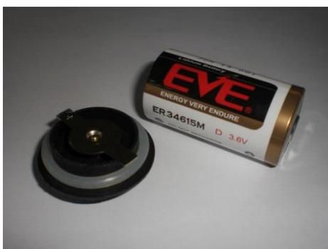
Figure 16: Battery from “EVE”, compartment cover
