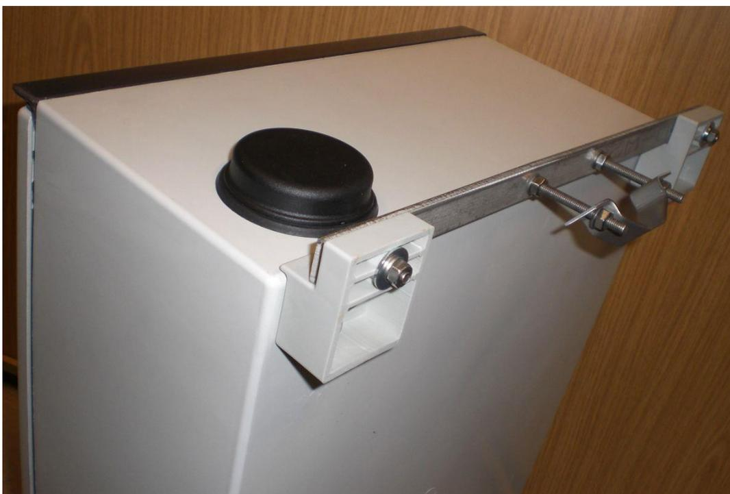
Figure 4: Coordinator housing with fixing rail (and mounted modem antenna)
