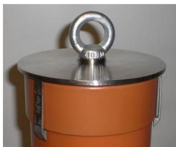
Figure 23: Pull-off tool for pipe lid
