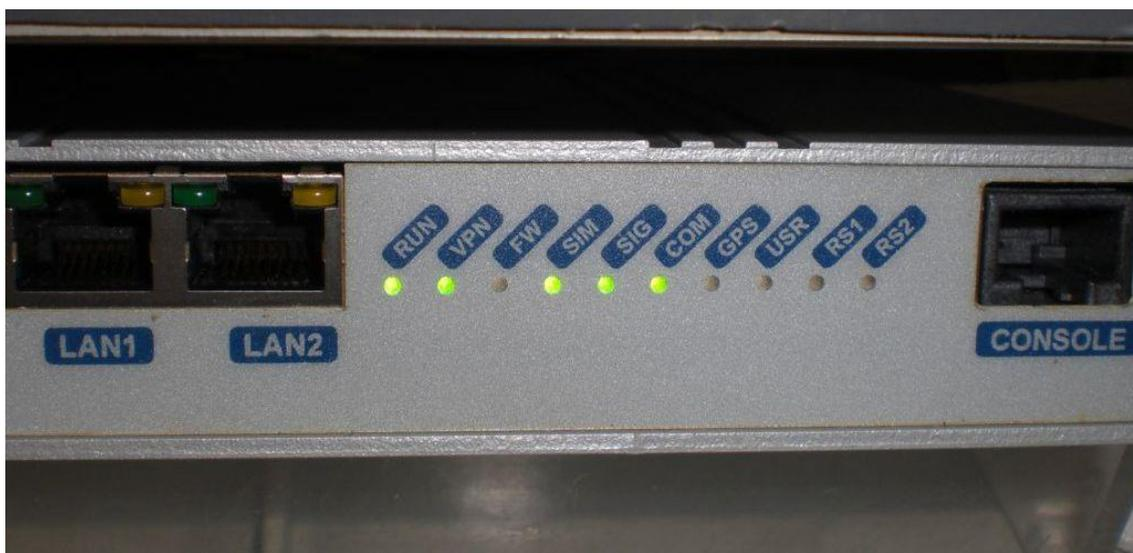
Figure 13: Signal LEDs of the OpenVPN modem during operation
