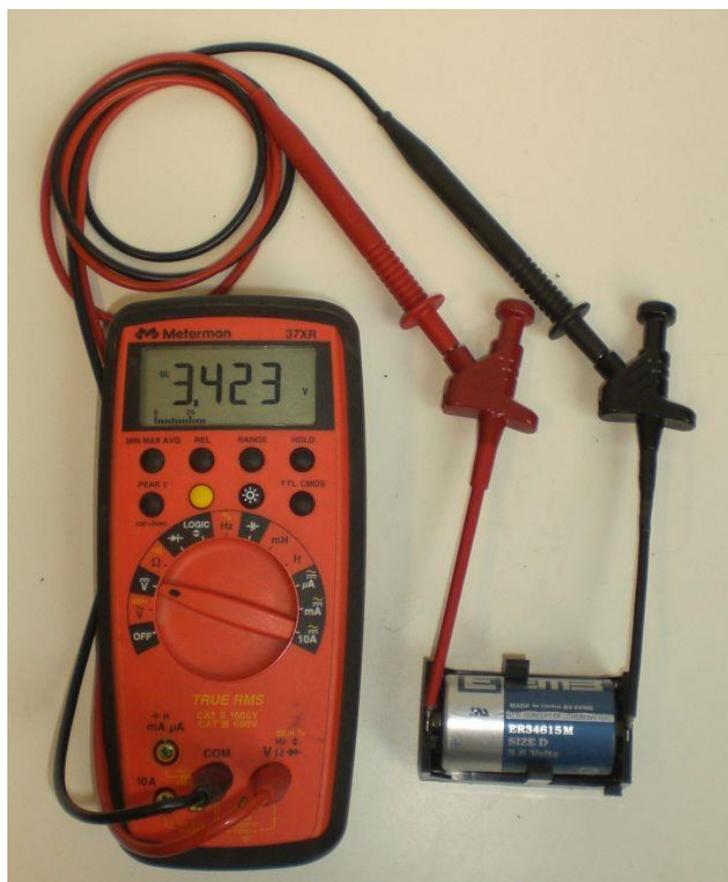
Figure 17: Measuring battery voltage with activating tool
