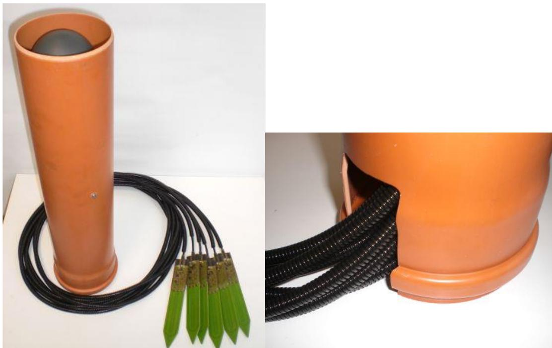
Figure 18: KG pipe with end device and cable opening
